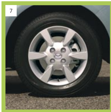
7 14" Alloy wheel, Design 43 6 spokes, tyre size 175/65 R14
